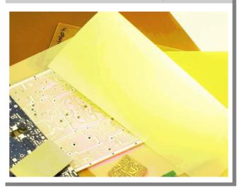
AD300A is a woven fiberglass reinforced PTFE/Microfine Ceramic composite material and is a significant improvement in cost/performance over traditional fluoropolymer-glass laminates. This combination offers designers an advantage for improving electrical performance through the use of advanced material without the additional cost traditionally associated with higher performance.
